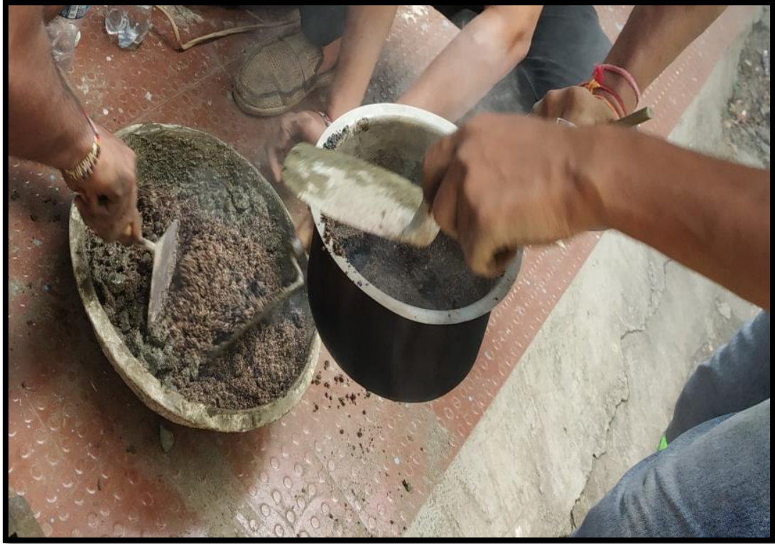
FIG-3: Mixing of sand cement aggregate and molten plastic
