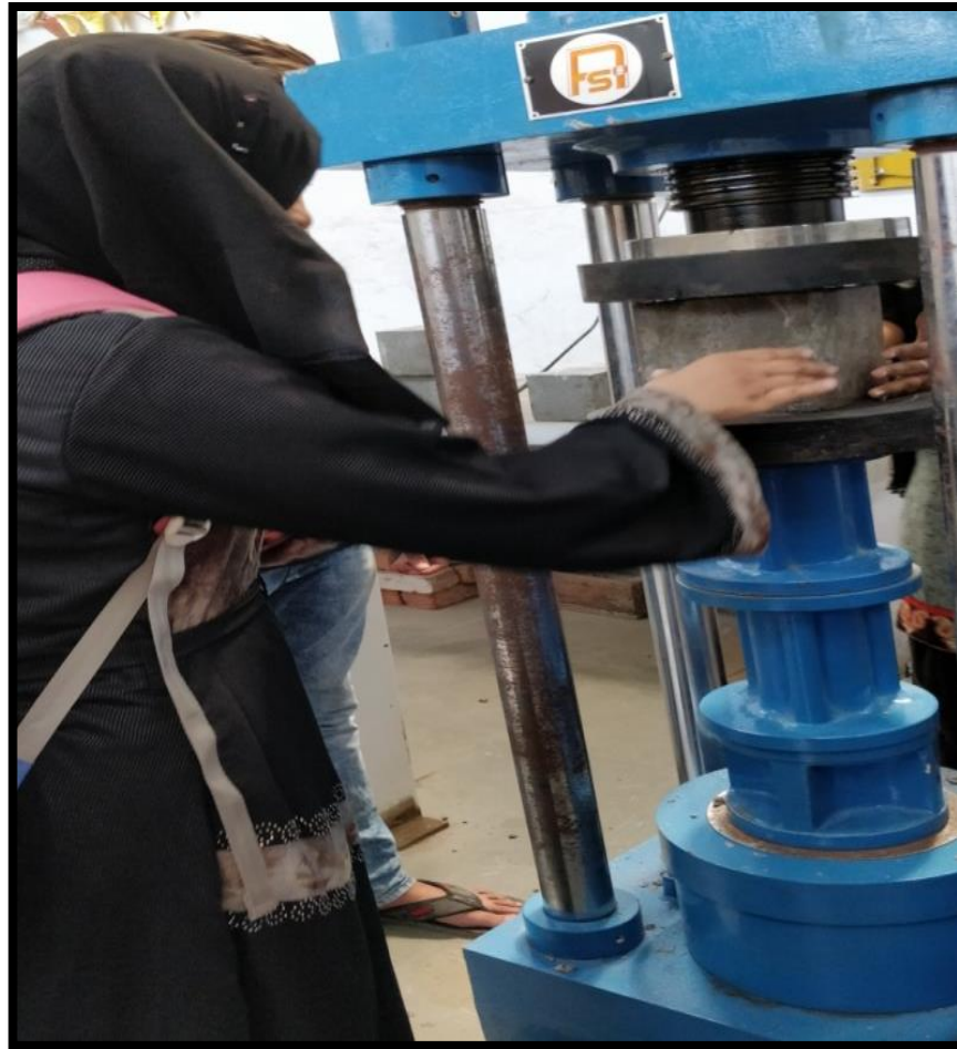
FIG-5: Testing of Cubes using compressive testing machine
