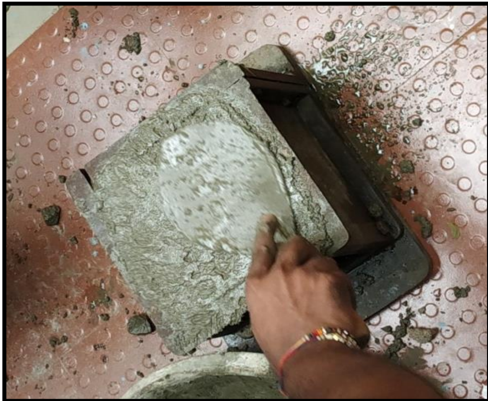
FIG-4: Casting of cubes
