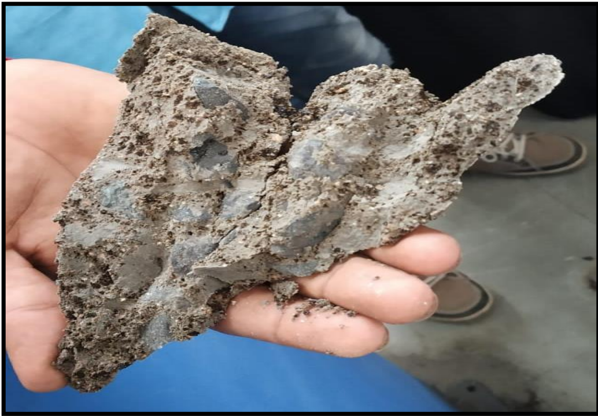
FIG-7: Internal structural matrix of plastic concrete cubes
