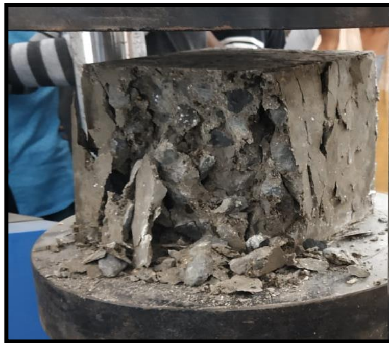
FIG-6: Failure pattern of Plastic concrete cubes
